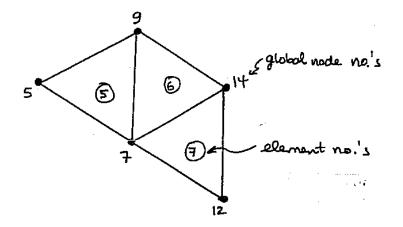
Procedure: Loop over the elements and sum local element matrices into "global" positions. Use element connectivity table to associate global with local node numbers for each element. Element Connectivity Table:
