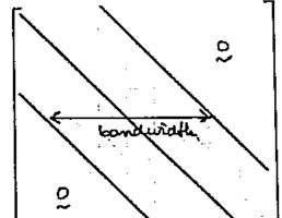
CE 60130 FINITE ELEMENT METHODS-LE 12|14 Bandwidth: maximum extent to within which nonzero locations are contained. Thus node numbering is extremely important to the efficiency of implementation of FE codes (assuming you're using banded matrix solvers).
